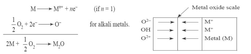
• During oxidation of a metal, metal oxide is formed as a thin film on the metallic surface which protects the metal from further corrosion.
